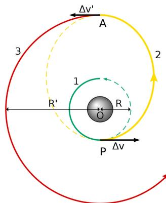
FIG. 3. Órbita de transferencia de Hohmann ([https://en.wikipedia.org/wiki/Hohmann\\_transfer\\_orbit#/media/File:Hohmann\\_transfer\\_modificada](https://en.wikipedia.org/wiki/Hohmann_transfer_orbit#/media/File:Hohmann_transfer_modificada)).
